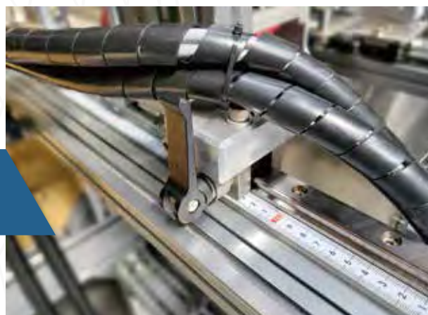
Ruler assists quickly move the print head modules to corrected position.
