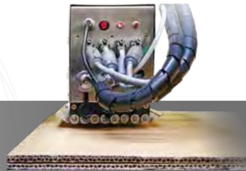
Print head elevation facility with figure meter for height adjustment reference.
