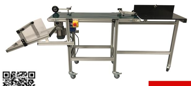
Stand Alone Machine for Feeding Pouches and Zippered Bags laying flat to allow for downstream printing and labeling.
