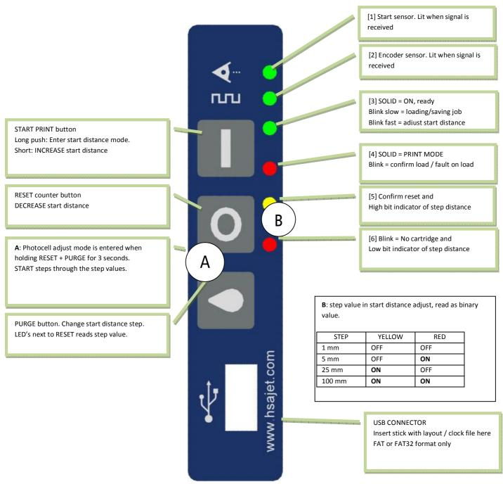
The MICRON provides signals to end users by LEDs. The meaning of LED signals are explained in the following pages.
