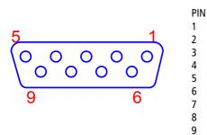
MEANING V ENC 5 V Not used EncB GND Not used 15 V Not used /EncB
