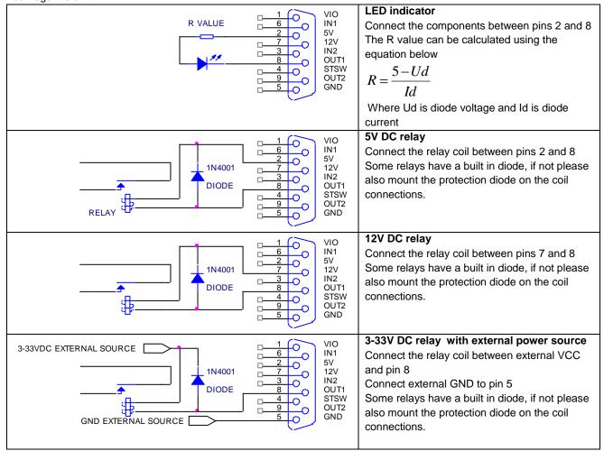
Warning: Do not connect a relay with a higher voltage than the voltage already connected to the VIO pin1 you will damage the unit.
