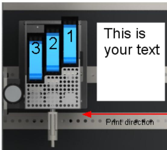
The offset distance of a print head is measured from the first nozzle row of the first pen in the head to the first nozzle row of the first pen in the previous print head.
