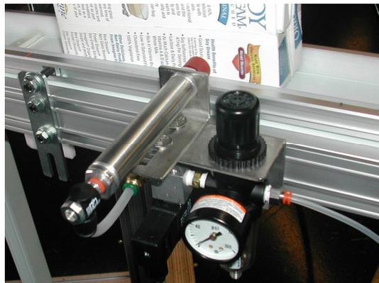
**Figure 6. Reject Mechanism Mounting**
