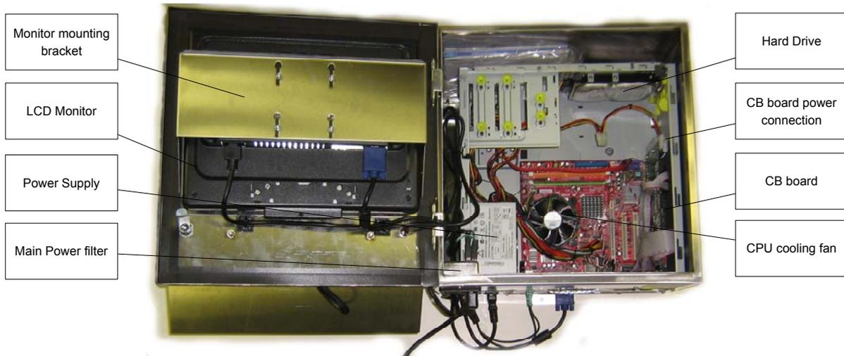
To remove the CB board you must remove the support mounting screw, power connection, ribbon cables and unlatch the yellow clamp.
