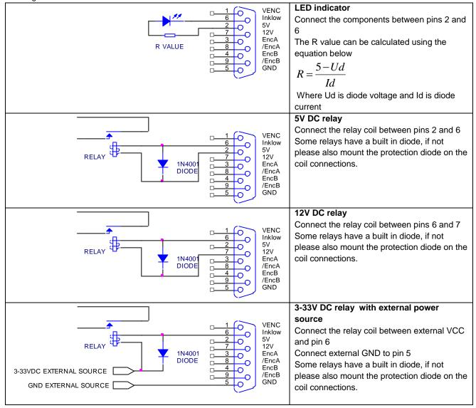
Warning: Do not connect a relay with a higher voltage than the voltage already connected to the VENC pin1 you will damage the unit.
