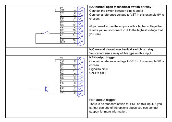
Warning: If you need to use the outputs with a higher voltage than 5 volts you must connect VST to the highest voltage that you use.
