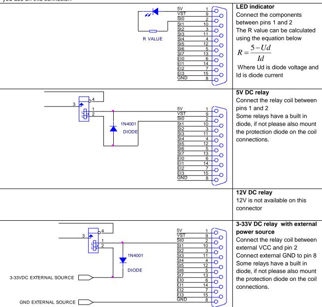
Warning: Do not connect a relay with a higher voltage than the voltage already connected to the VST pin 2 you will damage the unit. If you do not use the inputs on this connector you must connect VST to the highest voltage supply that you use on this connector.
