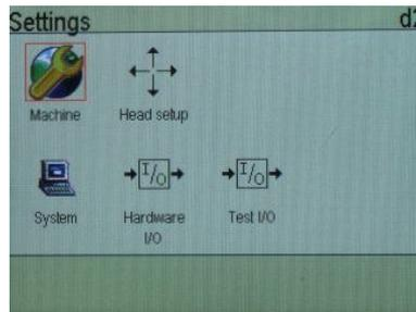
The MiniKey can use one or two physical heads, head 1 connected to the side, head 2 to the back, which each may be off, 1pen or 2pen. Inside head setup, choose the physical head to edit properties.
