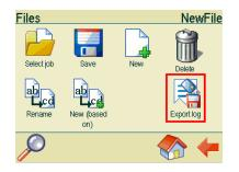
The extraction process is completed when the "busy symbol" is gone. The log files will be saved on the USB drive as LOGFILE.LOG for system events PRINTER.LOG for print data log
