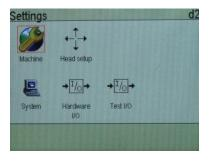
The MiniKey can use one or two physical heads, head 1 connected to the side, head 2 to the back, which each may be off, 1pen or 2pen. Inside head setup, choose the physical head to edit properties.
