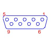
PIN Description VENC - voltage reference 5V Encoder A Encoder B GND Not used 12V /Encoder A (inverted) /Encoder B (inverted)
