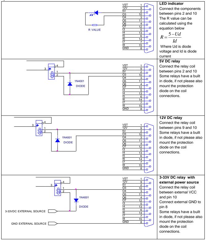
Warning: Do not connect a relay with a higher voltage than the voltage already connected to the VST pin 1 you will damage the unit. If you do not use the inputs on this connector you must connect VST to the highest voltage supply that you use on this connector.
