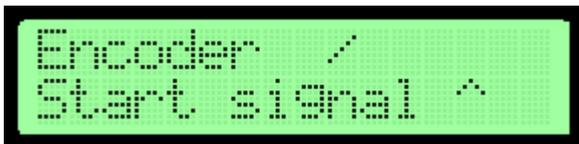
The encoder rotates the bar next to the word ( / | - \ ). Start signal switches between 2 arrows. ↑ = high, ↓ = low
