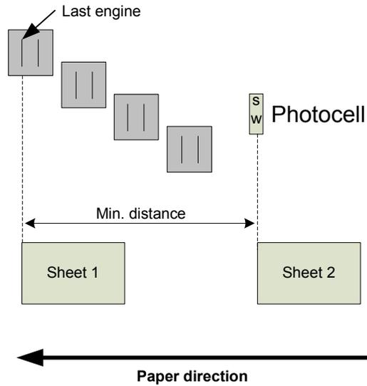
The distance between sheets (from front to front) is depending on the distance between the photocell and the last engine, because the last engine in the system must have started printing, when the photocell is triggered again. So formprint is NOT working under the minimum distance.
