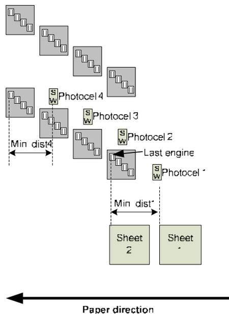
The minimum distance between sheets is different with extra Photocells, because this works as separate systems, so the last engine in the system is different. The limits in this system will be the longest distance from the Photocell to the corresponding last engine. In this system the best performance regarding minimum distance will be 4 Photocells.
