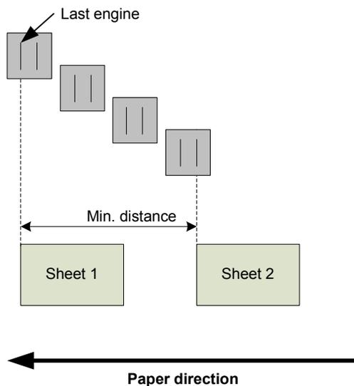
The distance between sheets (from front to front) is depending on the distance between the first engine and the last engine, because the last engine in the system must have started printing, when the first engine is starting printing the next picture. So formprint is NOT working under the minimum distance.
