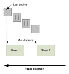
The distance between sheets(from front to front) is depending on the distance between the first engine and the last engine, because the last engine in the system must have started printing, when the first engine is starting printing the next picture.
