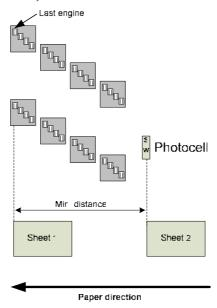
The distance between sheets(from front to front) is depending on the distance between the photocell and the last engine, because the last engine in the system must have started printing, when the photocell is triggered again.
