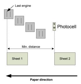
The distance between sheets(from front to front) is depending on the distance between the photocell and the last engine, because the last engine in the system must have started printing, when the photocell is triggered again.
