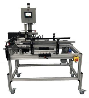
Stand Alone Machine to Pick and Place Pouches/Zippered Bags standing on edge for downstream printing and labeling
