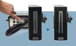
One button to purge and clean the print head nozzle, waste ink be collected automatically, maintain print quality in good condition and 100% mess-free.
