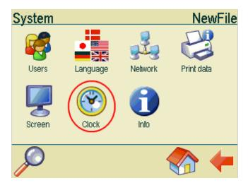
In the clock menu, enter current date, current time and settings for daylight saving time.
