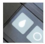
Purge button on each printhead From the printhead keypad, each cartridge can be purged individually. This minimizes ink wastage.
