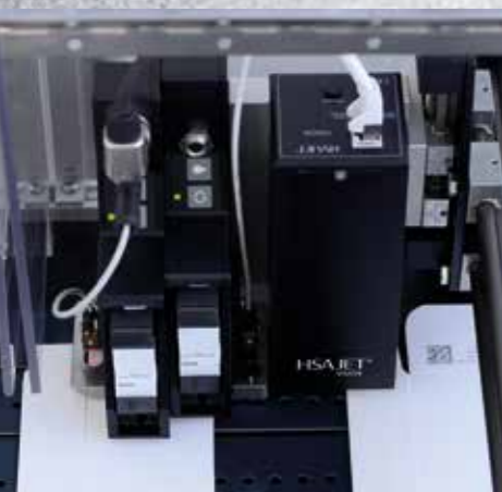
Camera and printhead on common bracket adjustable in height and across conveyor.
