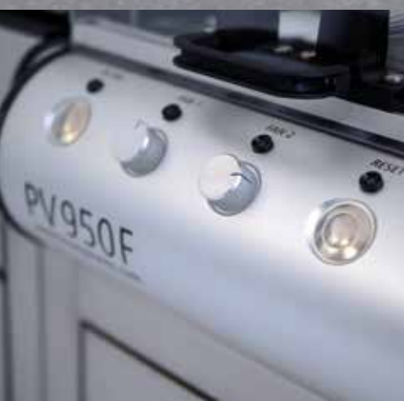
PC On, Emergency Stop, Reset and Fan buttons are placed on front of the machine.
