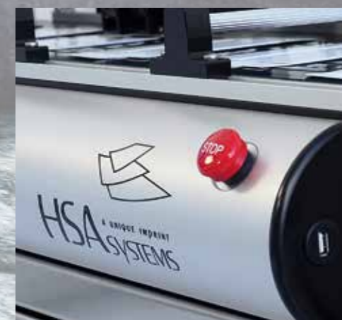
Emergency Stop is placed on front of the machine, right side.
